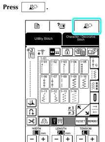
$\rightarrow\,$  The screen changes, and all keys and operation buttons are locked.
